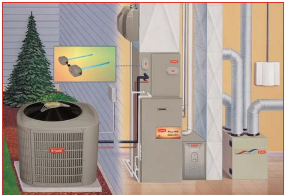
Air Conditioner and Gas Furnace System
